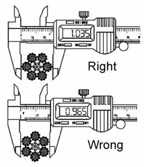
Right & wrong methods of measuring wire ropes
